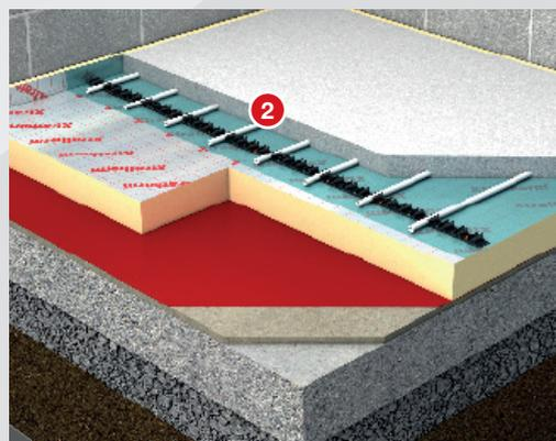
XT/UF provides the most efficient means of floor insulation. It has the strength and thermal properties required to reach the high performance U-Values asked for in the Building Regulations.
