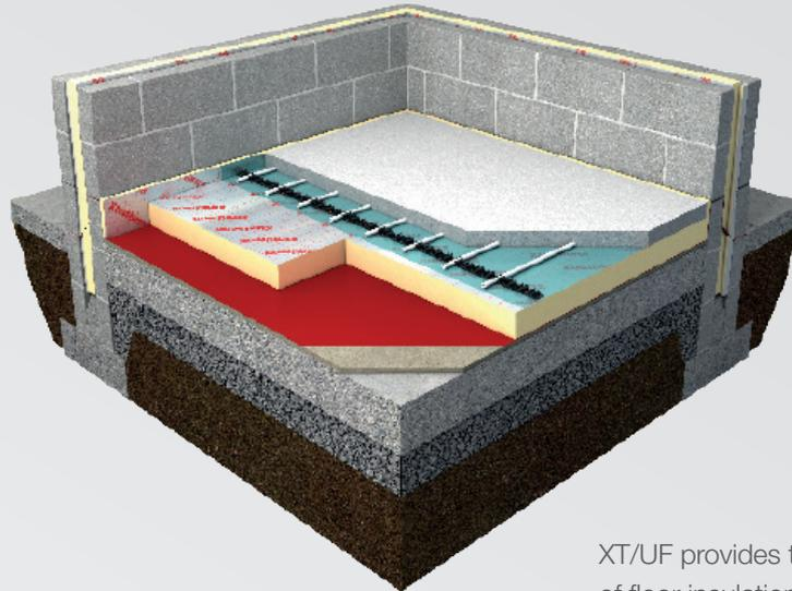
**1** Good detailing at the wall/floor junction is essential to reduce thermal bridging. By placing an upstand of Xtratherm Perimeter strip (XT/STR) insulation 25mm thick around the external and internal wall/floor junctions, a robust detail is created.
